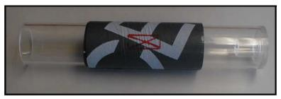
Figure 3-24: DMP-1 Material with Transducer Footprint Traced
